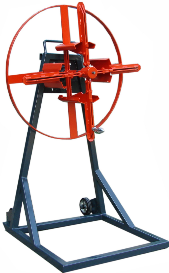
Manual winding machine with retractable front flange
